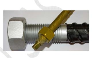
$oldsymbol{ \Theta}$  the thread resistance is weaker by 15 to 30% than the rod's
