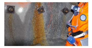
Choosing the right tube is essential to calibrate the ultimate load the bolt can support. Ex : for a head 46U there are 4 possible R32 tubes, from **210 to 360kN**.
