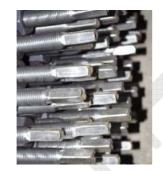
Forged square or flat parts to rotate the bolt
